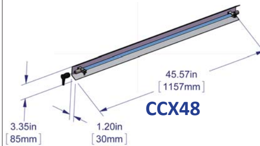
Photon Concentrator Focuses UV energy on coil
